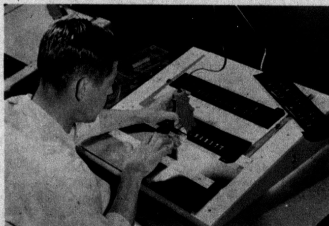
Fotosetter , one of several phototypesetting machines, externally resembles its hot metal counterpart, the Intertype slug-casting machine. But in place of the traditional metal pot, a camera is used. The operator has a choice of eight type sizes from a single photographic matrix. Lines of type are produced on sensitized paper or film instead of metal. ITU Training Center Instructor Alex Coleman, seated, explains it all to ANG President Arthur Rosnstock, left, Executive Vice President William J. Farson, center, and Director of Research and Information Ellis T. Baker.
