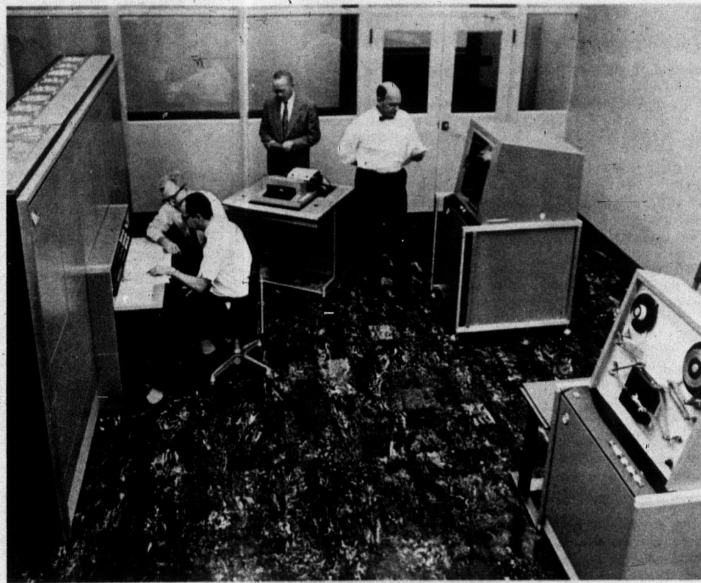
Reporter, above, perforates tape for the Los Angeles Times' new computer as he punches out his copy. His tape goes to the computer room, at right, where an electronic brain replaces the linotype operator. Copyreader's corrections are punched onto another tape on the electric typewriter in left center of the picture. The two tapes are fed into a high-speed reader, on the right, and a final tape, ready to be fed into an automatic typesetter, emerges from the high-speed punch in right center. The main section of the computer is on the left; it is activated by an operator sitting at the console.
